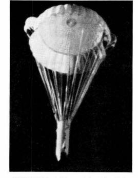
GUIDE FLAPS, visible on either side of the chute, are both open for neutral glide. The roll and glide flap system allows the cancellation of nearly 3000 feet of wind drift from a 15,000-foot drop.
